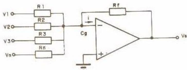
$$V_s = -((R_f/R_1)*V_1 + (R_f/R_2)*V_2 + \dots)$$
